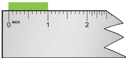
In this second case (sketch above), it is apparent that the object is, as nearly as we can read, 1 inch. Since we know the tenths place is zero and can estimate the hundredths place to be zero, the measurement should be reported as 1.00 inch. It is vital that you include the zeros in your reported measurement because these are measured places and are significant figures.
