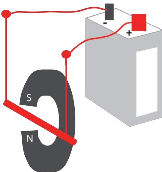
In the sketch above, a circuit is connected to a battery, with one part of the circuit placed inside a magnetic field. When current runs through the circuit, a force will be exerted on the wire by the magnetic field, causing the wire to
