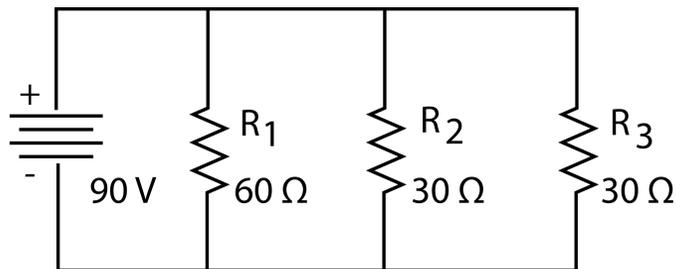
The current through each resistor can be found using the voltage drop and the resistance of that resistor:
