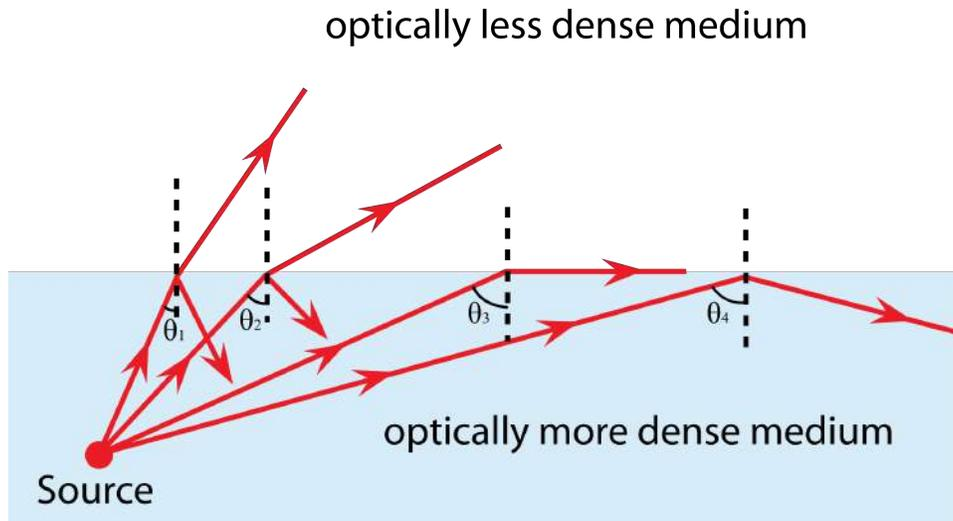
Consider a ray of light passing from water into air. The index of refraction for air is 1.00 and for water is 1.36. Using Snell's Law,  $n_i \sin \theta_i = n_r \sin \theta_r$ , and allowing the angle of refraction to be  $90^\circ$ , we can solve for the angle of incidence which would cause the light ray to stay in the old medium.
