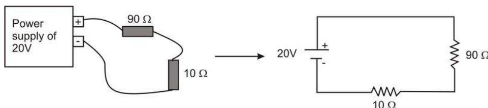
Both resistors are in the same 'river', so both have the same current flowing through them. Neither resistor has a direct connection to the power supply so neither has 20V across it. But the combined voltages across the individual resistors add up to 20V.
