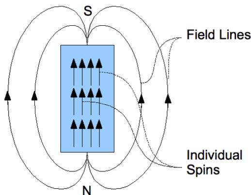
If we were to cut the magnet above in half, it would still have north and south poles; the resulting magnetic field would be qualitatively the same as the one above (but weaker).
