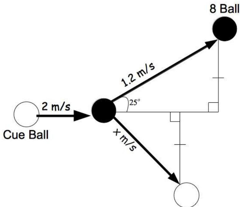
We know that the momentum in the y direction of the two balls is equal. Therefore we can say that the velocity in the y direction is also equal because the masses of the two balls are equal.
