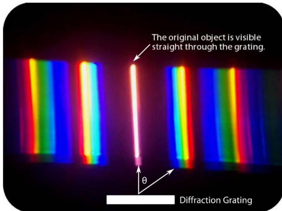
Also in this image is the measurement for  $\theta$ , which can be used to calculate the wavelength of the original light source. The equation from the double slit experiment can be adjusted slightly to work with diffraction gratings. Where  $\lambda$  is the wavelength of light,  $d$  is the distance between the slits on the grating, and  $\theta$  is the angle between the incident (original) light and the refracted light,
