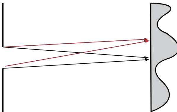
Just as in double slit interference, a pair of similar triangles can be constructed in the interference pattern. The pertinent values from these triangles are the width of the slit,  $w$ , the wavelength,  $\lambda$ , the distance from the central bright spot to the first dark band,  $x$ , and the distance from the center of the slit to back wall,  $L$ . The relationship of these four values is
