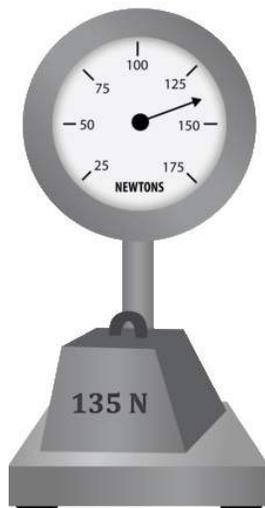
Weight is measured in force units which is Newtons in the SI system. The weights measured for an object would not be the same on the earth and moon because the gravitational field on the surface of the moon is one-sixth of the magnitude of the gravitational field on the surface of the earth.
