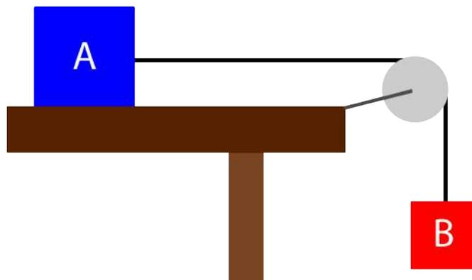
**Solution:** The force tending to move the system is the weight of box B and the force resisting the movement is the force of friction between the table and box A. The mass of the system would be the sum of the masses of both boxes. The acceleration of the system will be found by dividing the net force by the total mass.
