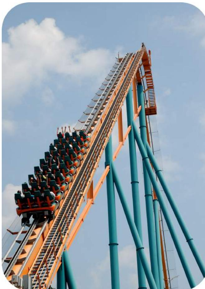
In order for the roller coaster to run down the incline by gravitational attraction, it first must have work done on it towing it up to the top of the hill. The work done on the coaster towing it to the top of the hill becomes potential energy stored in the coaster and that potential energy is converted to kinetic energy as the coaster runs down from the top of the hill to the bottom.
