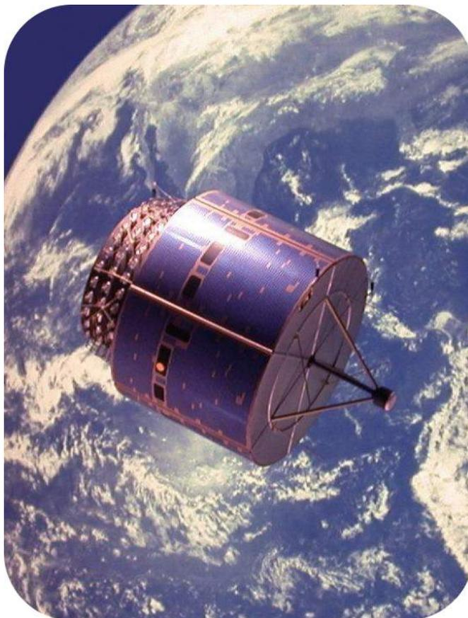
Weather satellites, like the one shown above, are found miles above the earth's surface. Satellites can be polar orbiting, meaning they cover the entire Earth asynchronously, or geostationary, in which they hover over the same spot on the equator.
