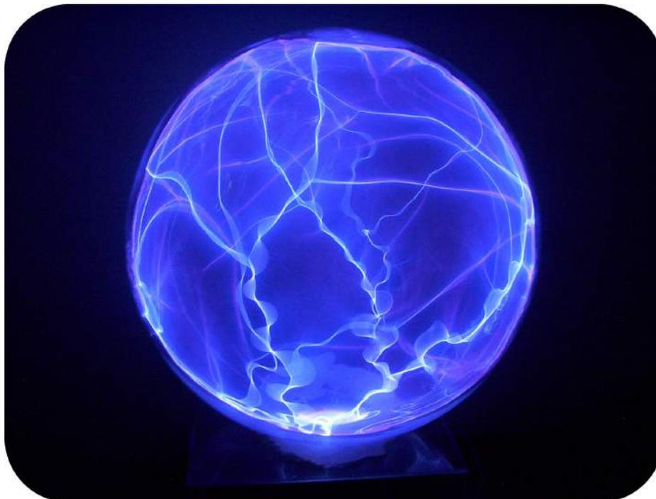
A plasma globe, such as the one pictured above, is filled with a mixture of noble gases and has a high-voltage electrode at the center. The swirling lines are electric discharge lines that connect from the inner electrode to the outer glass insulator. When a hand is placed on the surface of the globe, all the electric discharge travels directly to that hand.
