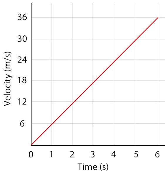
In displacement versus time graphs, the slope of the line is the velocity of the object and in this case of velocity versus time graph, the slope of the line is the acceleration. If you take any segment of this line and determine the  $\Delta y$  to  $\Delta x$  ratio, you will get  $6.0 \text{ m/s}^2$  which we know to be the constant acceleration of this object.
