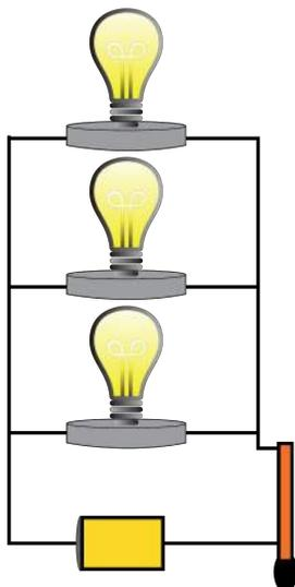
In the design of this parallel circuit, each resistor (light bulb) is connected across the battery as if the other two resistors were not present. Remember that the current going through each resistor goes through only the one resistor. Therefore, the voltage drop across each resistor must be equal to the total voltage drop through the circuit.
