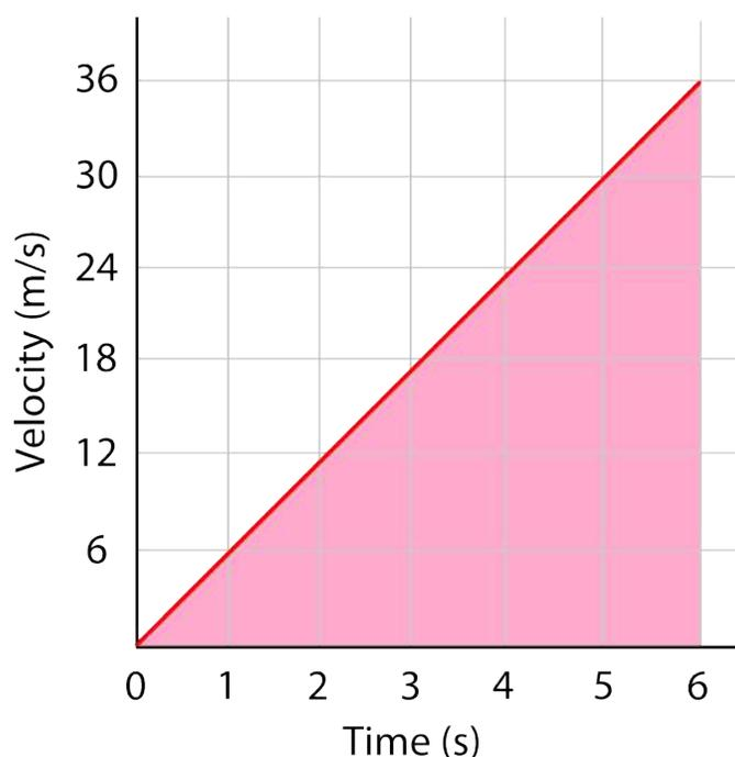
The area of this triangle would be calculated by  $\text{area} = \left(\frac{1}{2}\right) (6.0 \text{ s})(36 \text{ m/s}) = 108 \text{ m}$ .
