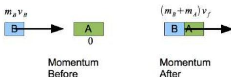
**Solution** : To find mass of block B we have a simple subtraction problem. We know that the combined mass is 10kg and the mass of block A is 8.0kg.
