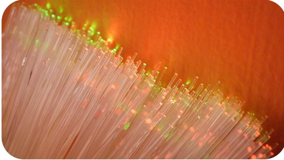
Total internal reflection allows the light to travel down the optical fiber and not pass through the sides of the tube. The light continuously reflects from the inside of the tube and eventually comes out the end. Optical fibers make interesting lamps but they are also used to transport telephone and television signals.
