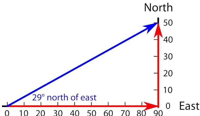
If we are using totally graphic means of adding these vectors, the magnitude of the sum would be determined by measuring the length of the sum vector and comparing it to the original standard. We would also use a compass to measure the angle of the summation vector.
