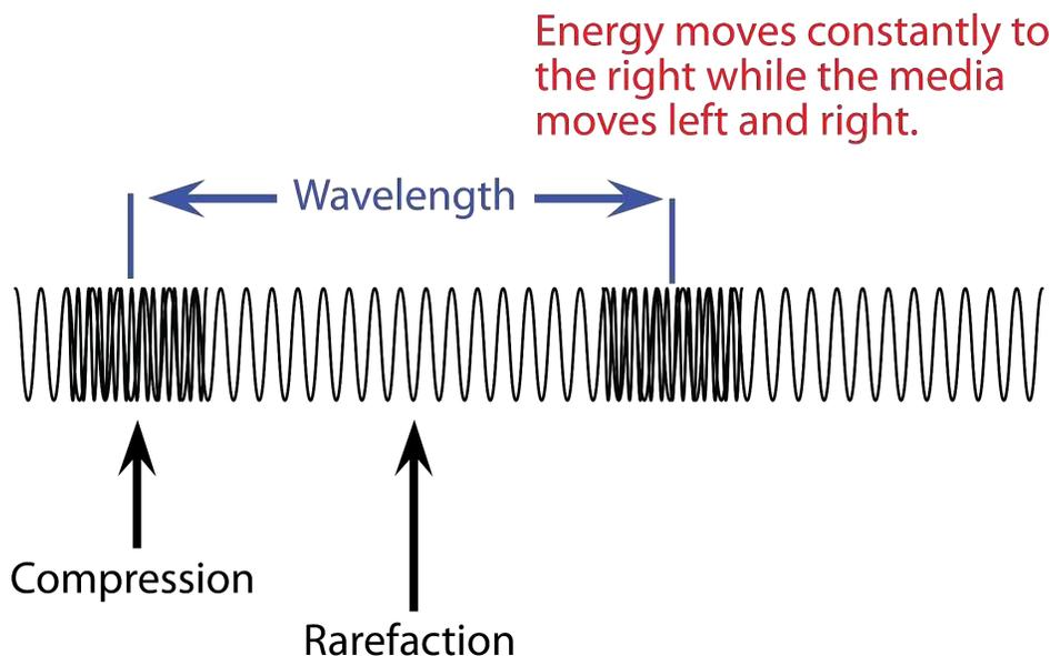
**Example Problem:** A sonar signal (sonar is sound waves traveling through water) of  $1.00 \times 10^6$  Hz frequency has a wavelength of 1.50 mm in water. What is the speed of sound in water?
