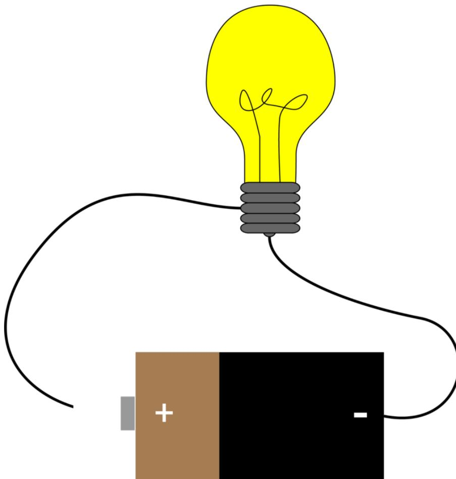
Jose made this sketch of a battery and light bulb for science class. If this were a real set up, the light bulb wouldn't work. The problem is the loose wire on the left. It must be connected to the positive terminal of the battery in order for the bulb to light up.
