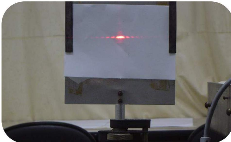
Though it looks like a double slit interference pattern, the pattern on the screen are actually the results of light diffracting through a single slit with the ensuing interference.
