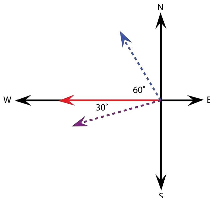
Since momentum is conserved in this collision, the sum of the momenta of balls  $A$  and  $B$  after collision must be  $10.0 \text{ kg m/s}$  west.
