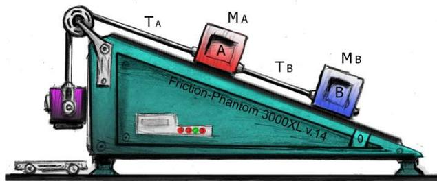
The pulley at the top of the incline is massless and frictionless. The larger mass,  $M$ , is accelerating downward with a measured acceleration  $a$ . The smaller masses are  $m_A$  and  $m_B$ ; the angle of the incline is  $\theta$ , and the coefficient of kinetic friction between each of the masses and the incline has been measured and determined to be  $\mu_K$ .
