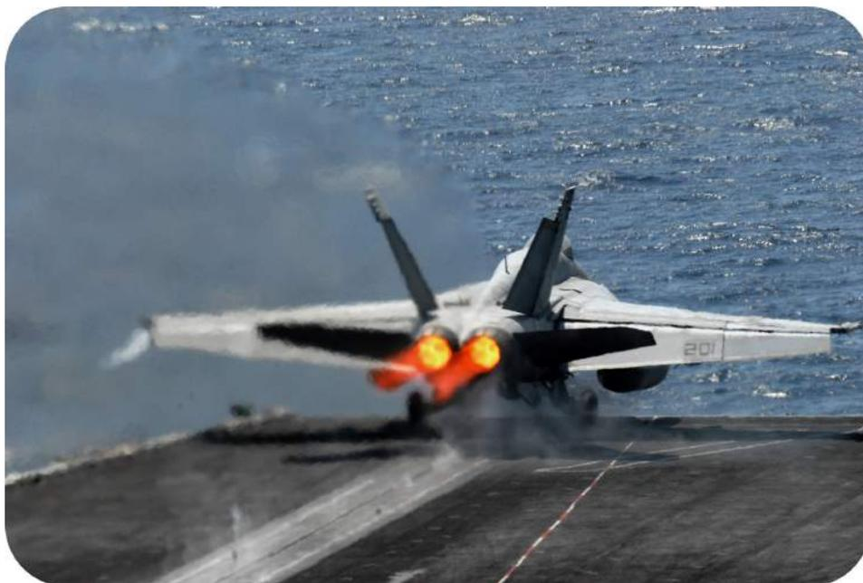
This military jet requires a tremendous amount of work done on it to get its speed up to takeoff speed in the short distance available on the deck of an aircraft carrier. Some of the work is done by the plane's own jet engines but work from a catapult is also necessary for takeoff.
