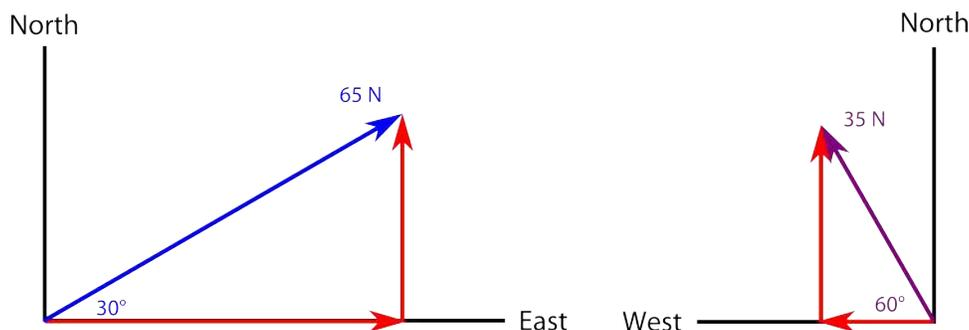
We can resolve each of the vectors into two components. The components are on the axes lines. The **resolution of vectors** reduces each vector to a component on the north-south axis and a component on the east-west axis.
