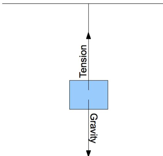
If the object is in equilibrium, tension must be equal in magnitude and opposite in direction to gravity. This force transfers the gravity acting on the object to whatever the wire or string is attached to; in the end it is usually a Normal Force — between the earth and whatever the wire is attached to — that ends up balancing out the force of gravity on the object.
