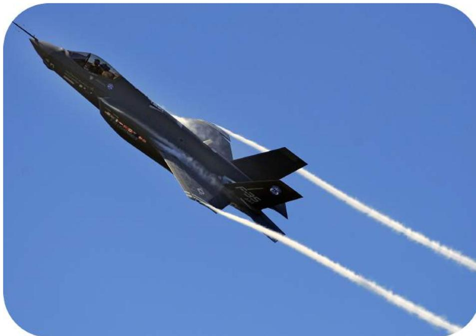
Wingtip vortices are often thought to be a type of contrail but are actually produced from a different process. During very specific weather conditions you may see vapor trails form at the rear of the wingtips of jet aircraft on takeoff or landing. This phenomenon occurs due to a decrease in pressure and temperature as the wing generates lift.
