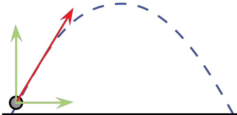
**Example Problem:** A cannon ball is fired with an initial velocity of 100. m/s at an angle of  $45^\circ$  above the horizontal. What maximum height will it reach and how far will it fly horizontally?
