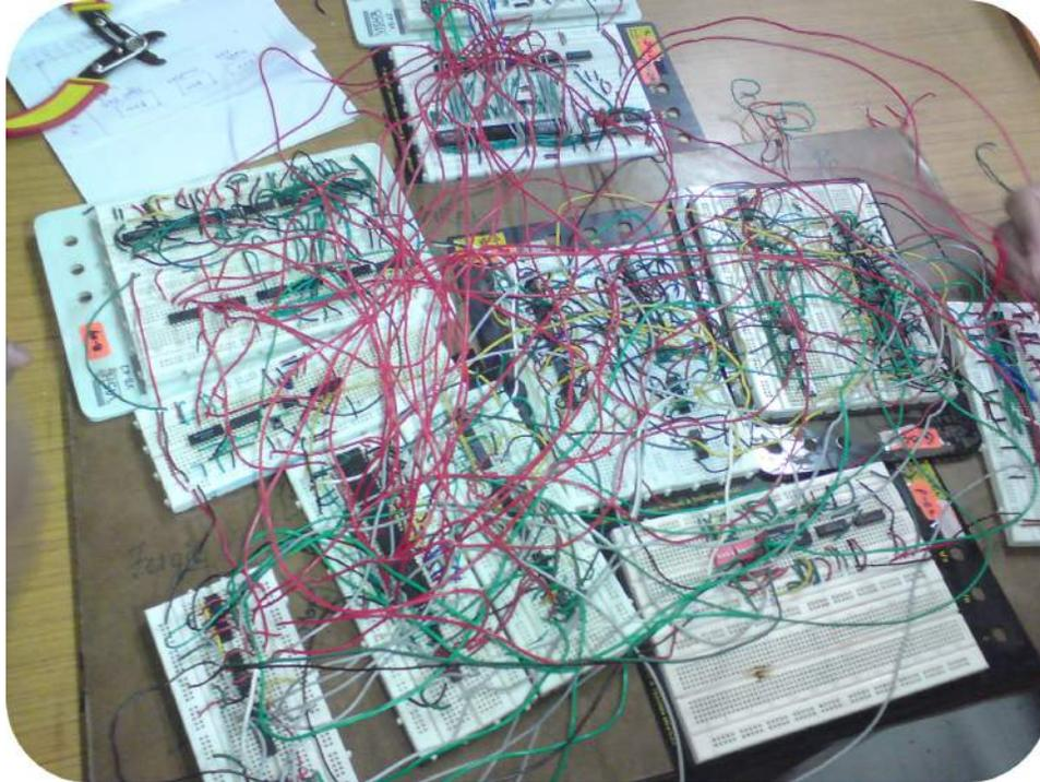
Electrical circuits can become immensely complicated. This circuit is a polynomial plotter, which allows users to plot polynomials and evaluate functions at various  $x$  values.
