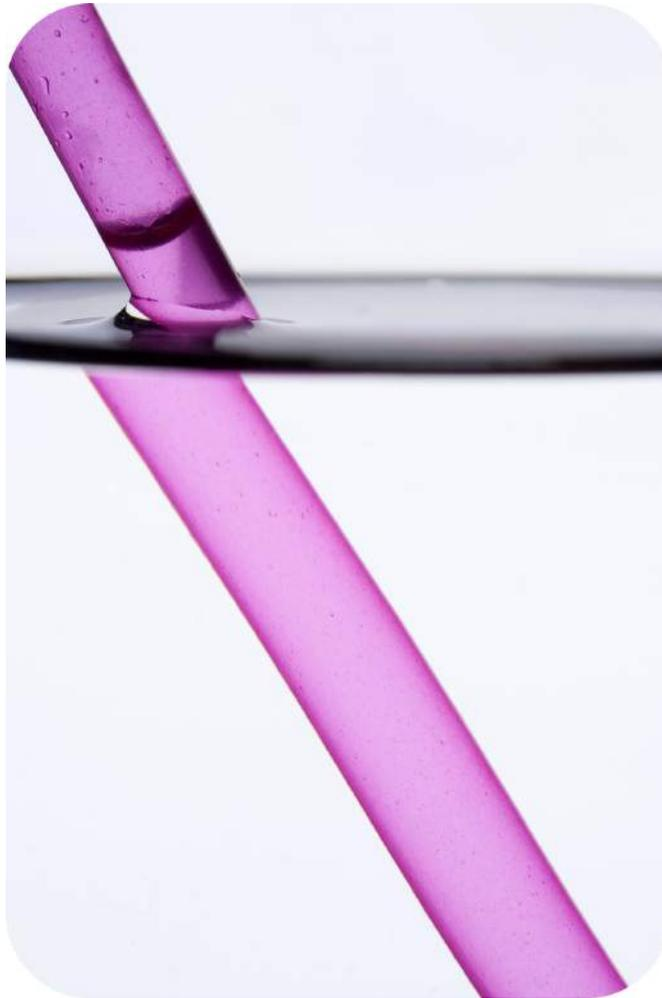
A straw in a glass of water seen from the side often appears broken, even though it is not. The apparent break is due to the bending of light rays leaving the straw; as the light passes from the water to the glass and from the glass to the air, the light rays are bent. Nonetheless, your eye traces the light ray backward as if the light has followed a straight path from its origin at the straw. Since the light appears to have come from a different place, your eye sees the straw as being broken.
