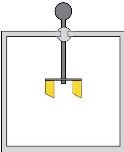
When a negatively charged object is brought near the knob of a neutral electrostatic test tube, the negative charge repels the electrons in the knob, and those electrons move down the stem into the leaves. Excess electrons flow from the rod into the ball, and then downwards making both leaves negatively charged. Since both leaves are negatively charged, they repel each other. When the rod is removed, the electrostatic test tube will remain charged because of the extra electrons added to it.
