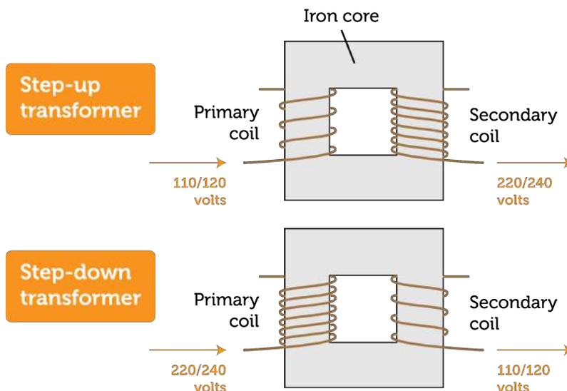
$$\frac{\text{secondary voltage}}{\text{primary voltage}} = \frac{\text{number of turns on secondary}}{\text{number of turns on primary}}$$
