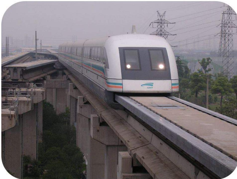
Some countries are using powerful electromagnets to develop high-speed trains, called maglev, or magnetic levitation, trains. These trains use the repulsive force of magnets to float over a guide way, removing the friction of steel wheels and train tracks. Reducing this friction allows the trains to travel at much higher speeds.
