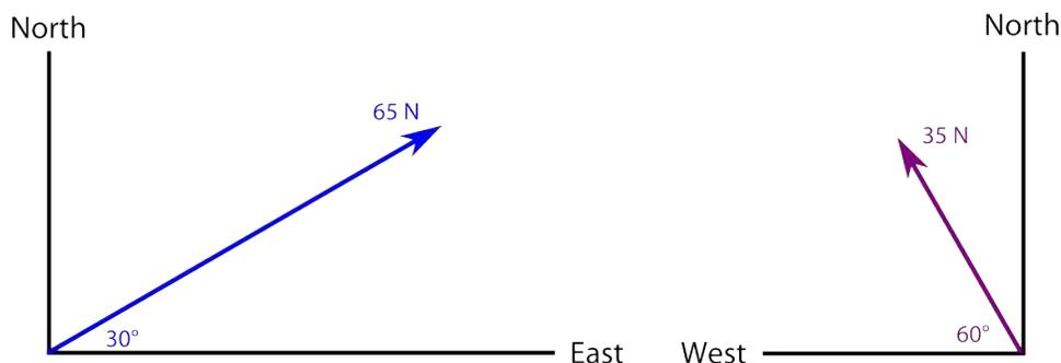
The two vectors we are to add is a force of 65 N at 30° north of east and a force of 35 N at 60° north of west.
