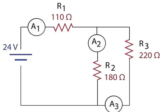
**Solution:** We start by simplifying the parallel resistors  $R_2$  and  $R_3$ .
