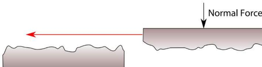
With the bumps, lumps, and imperfections emphasized as in the image above, it becomes more apparent that if we try to slide the top block over the lower block, there will be collisions involved when bumps impact on bumps. The forward motion causes the collisions with bumps which then exert a force in opposite way the block is moving. The force of friction always opposes whatever motion is causing the friction.
