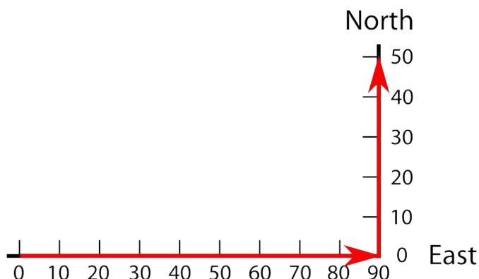
The graphical process for adding vectors in two dimensions is to place the tail of the second vector on the arrow head of the first vector as shown above.
