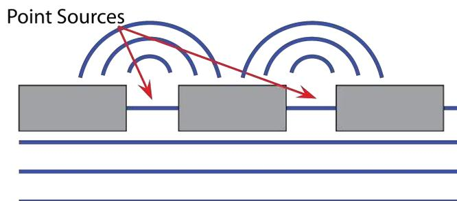
As long as these two circular waves have the same wavelength, they interfere constructively and destructively in a specific pattern. This pattern is called the **wave interference pattern** and is characterized by light and dark bands. The light bands are a result of constructive interference, and the dark bands occur because of destructive interference.
