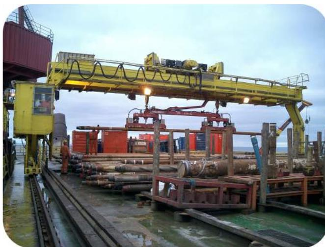
The overhead portion of this machine (painted yellow) is a lifting electromagnet. It is lowered to the deck where steel pipe is stored and it picks up a length of pipe and moves it to another machine where it is set upright and lowered into an oil well drill hole.
