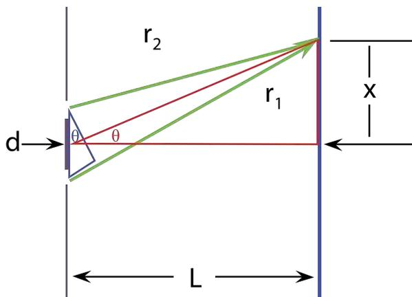
$r_1$  and  $r_2$  are the distances from the slits to the first order fringe. We know that the fringes are a result of constructive interference, and that the fringe is a result of the crest of two waves interfering. If we assume that  $r_2$  is a whole number of wavelengths (confirm for yourself that this is a logical assumption), then  $r_1$  must be one more wavelength. This is because  $r_1$  and  $r_2$  are the distances to the first order fringe. Mathematically, we can let
