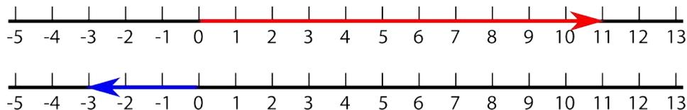
The red vector has a magnitude of 11 in the positive direction on the number line. The blue vector has a magnitude of -3 in the negative direction on the number line. In order to add these two vectors, we place one of the vectors on a number line and then the second vector is placed on the same number line such that its origin is on the arrow head of the first vector.
