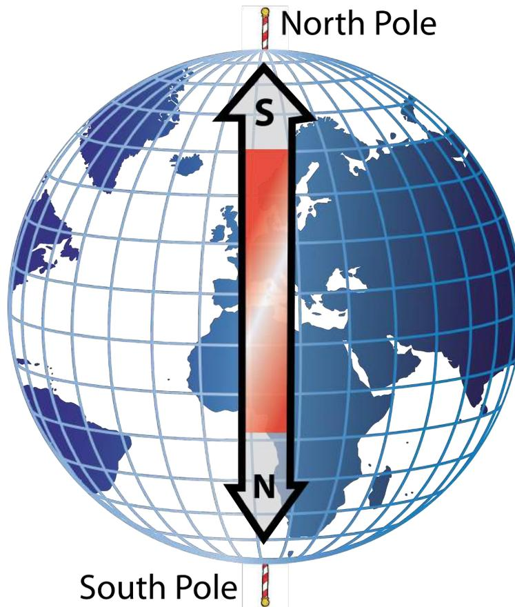
The Earth's geographic north pole (which is close to, but not exactly at the magnetic pole) attracts the north poles of magnets. We know, therefore, that this pole is actually the Earth's magnetic south pole. This can be seen in the image above; the geographic north and south poles are labeled with barber shop poles, and the Earth's **magnetic poles** are indicated with the double-headed arrow.
