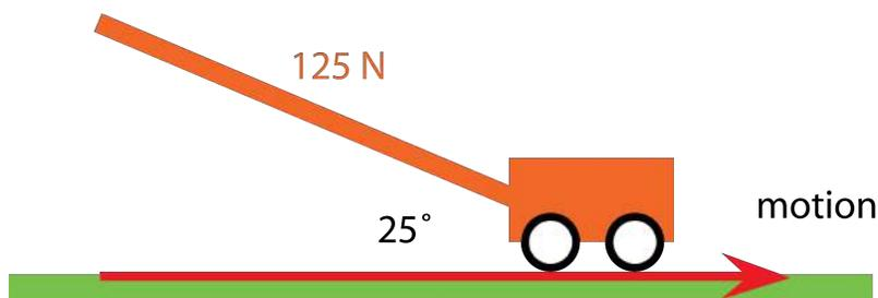
**Solution:** The solution requires that we determine the component of the force that was in the direction of the motion of the lawnmower. The component of the force that was pushing down on the ground does not contribute to the work done.
