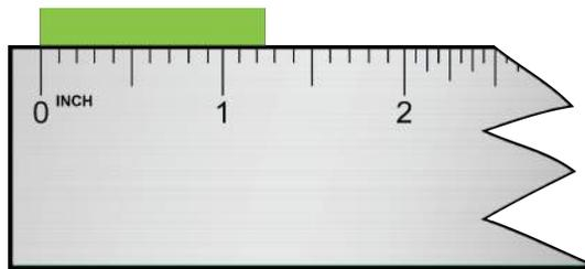
In the sketch shown above, the correct measurement is greater than 1.2 inches but less than 1.3 inches. It is proper to estimate one place beyond the calibrations of the measuring instrument. This ruler is calibrated to 0.1 inches, so we can estimate the hundredths place. This reading should be reported as 1.25 or 1.26 inches.
