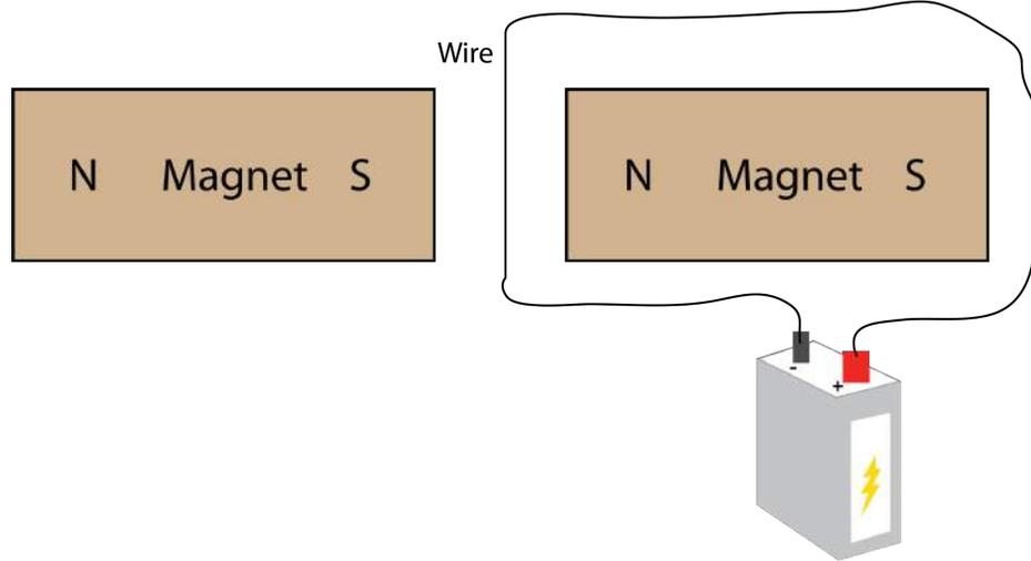
2. Which way will the coil spin when current passes through the wire?
