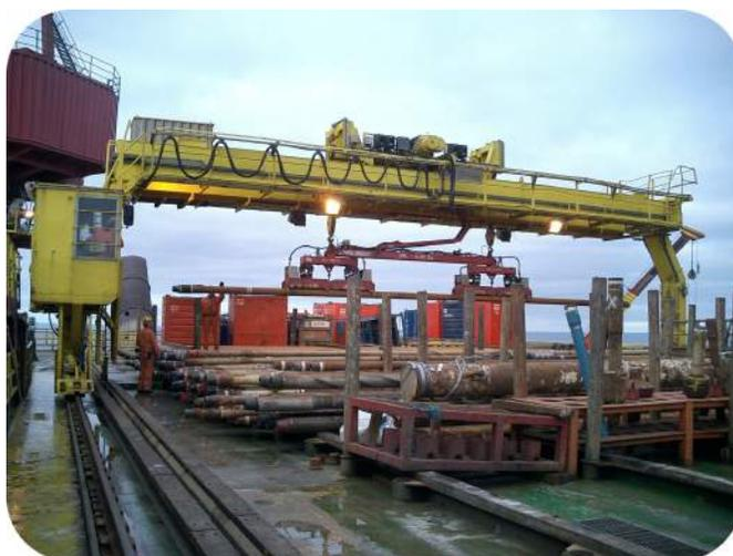
The overhead portion of this machine (painted yellow) is a lifting electromagnet. It is lowered to the deck where steel pipe is stored and it picks up a length of pipe and moves it to another machine where it is set upright and lowered into an oil well drill hole.
