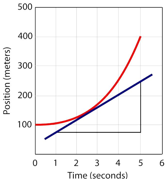
In the image above, the red line is the position vs time graph and the blue line is an approximated slope for the line at  $t = 2.5$  seconds. The rise for this slope is approximately 170 m and the time interval (run) is 4.0 seconds. Therefore, the approximated slope is 43 m/s.
