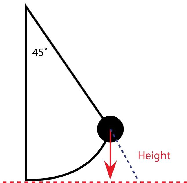
**Solution:** You can use trigonometry to find the vertical height of the ball in the pulled back position. This vertical height is found to be 0.877 m.
