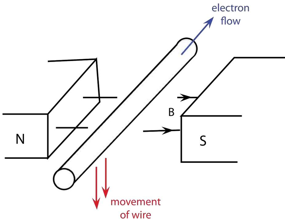
This process allows us to convert mechanical energy (the motion of the wire) into electrical energy (the current). This is the opposite of what happens in an electric motor where electrical energy is converted into mechanical energy.
