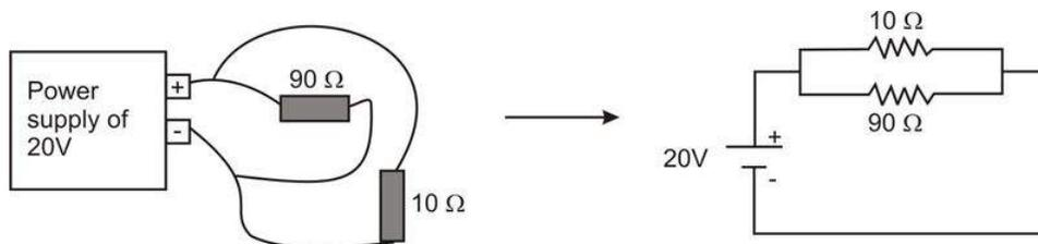
Both resistors are directly connected to the power supply, so both have the same 20V across them. But they are on different 'rivers' so they have different current flowing through them. Lets go through the same questions and answers as with the circuit in series.
