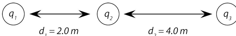
$$\text{Solution: } F_e = \frac{Kq_1q_2}{d^2} = \frac{(9.0 \times 10^9 \text{ N}\cdot\text{m}^2/\text{C}^2)(10.0 \times 10^{-6} \text{ C})(2.0 \times 10^{-6} \text{ C})}{(2.0 \text{ m})^2} = 0.045 \text{ N (towards } q_3)$$
