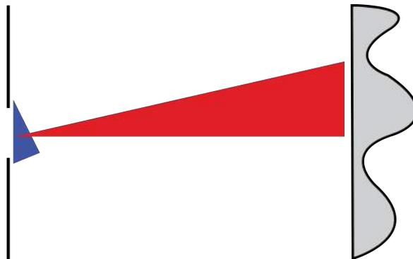
**Example Problem:** Monochromatic light of wavelength 605 nm falls on a slit of width 0.095 mm. The slit is located 85 cm from a screen. How far is the center of the central bright band to the first dark band?
