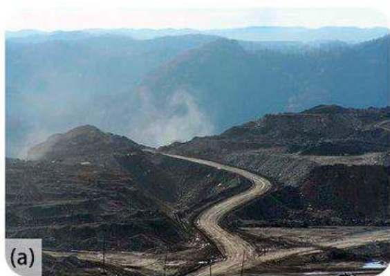
(a) Coal being mined by mountaintop removal.
